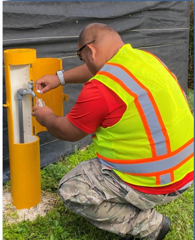
Gabriel Dela Cruz collects a water sample from a CUC tap to be tested for the bacteria total coliform and E. coli . Monthly testing of the water for chlorine and bacteria helps CUC Rota ensure that the water we deliver to our customers is safe to drink.
