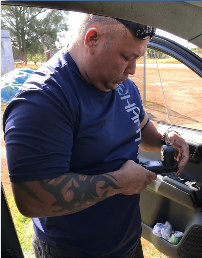
Peter Taitano measures the amount of chlorine in a CUC Rota water sample. Every day, water operators check several sites throughout the CUC Rota water system to ensure that all areas have the proper amount of chlorine.
