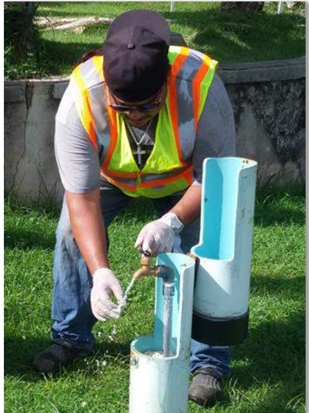
Water Operator, John Sablan, measures chlorine at a sample tap. Every day, water operators check several sites throughout the CUC Tinian water system to ensure that all areas have the proper amount of chlorine.
